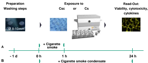
Figure 1: Experimental setup for submerge exposure to Csc for 24 h (B) and for exposure of lung tissue to cigarette smoke at ALI (A).
