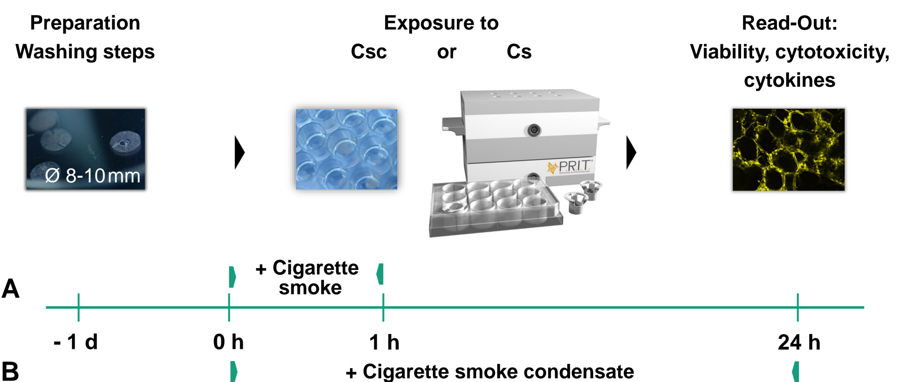
Fig. 1: Experimental setup for submerge exposure to Csc for 24 h (B) and for exposure of lung tissue to cigarette smoke at ALI (A).
