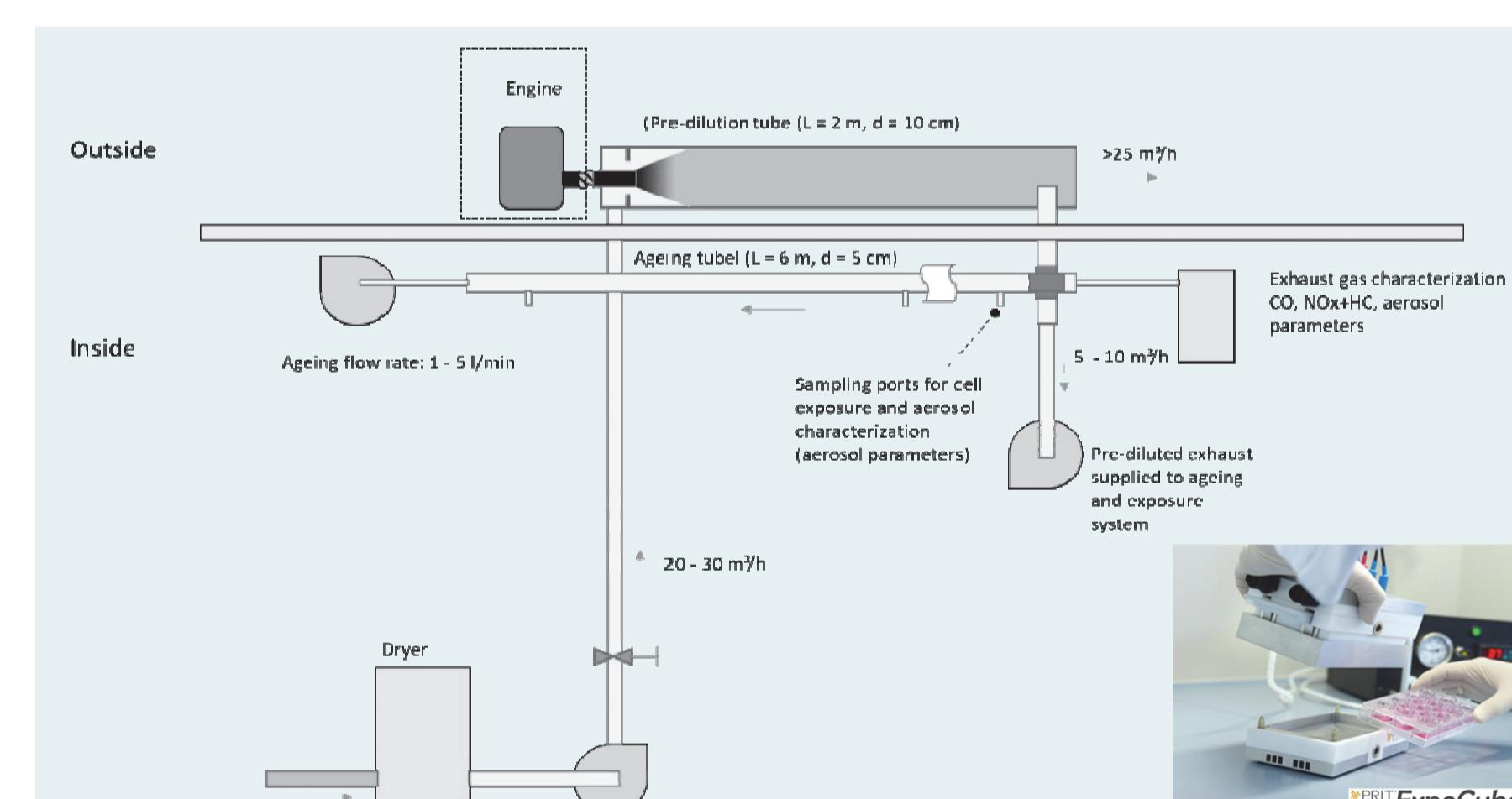
Figure 1: Experimental set-up for generation of complex test atmospheres for nano-particle dose-metric studies. Taking advantage of Brownian coagulation, number dose can be varied independently from mass dose.
