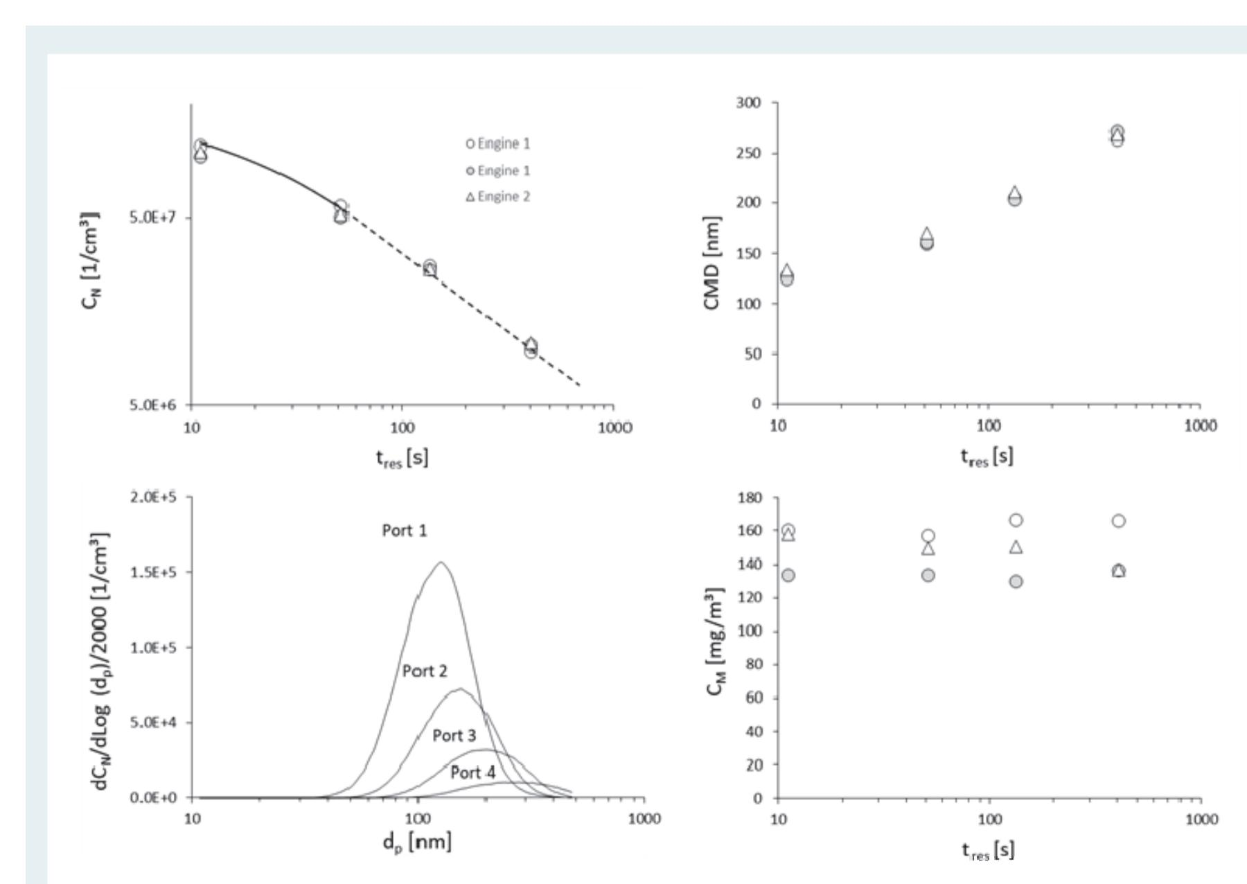
Figure 2: Aerosol properties at the sampling ports representing different stages of ageing: number concentration, count mean diameter, number distribution density (SMPSS-measurements), and mass concentration (gravimetric analysis).
