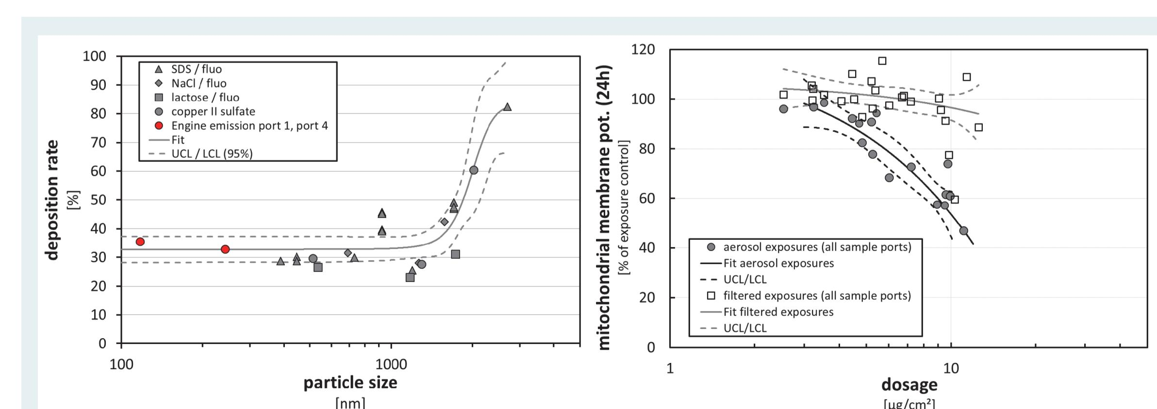
Figure 3: Deposition analysis using Mo-spiked engine exhaust in comparison to historical results (P.R.I.T.® ExpoCube®) (left). Cell exposures to aerosols from all sample ports using filtered (gas-phase) or non-filtered aerosol (right).
