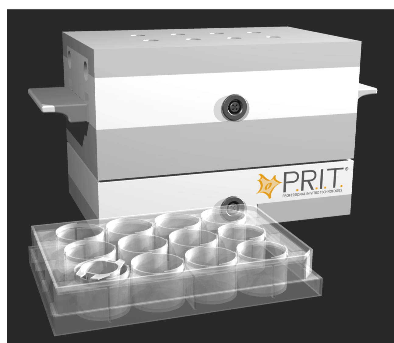
Figure 2 Exposure device "ExpoCube"
